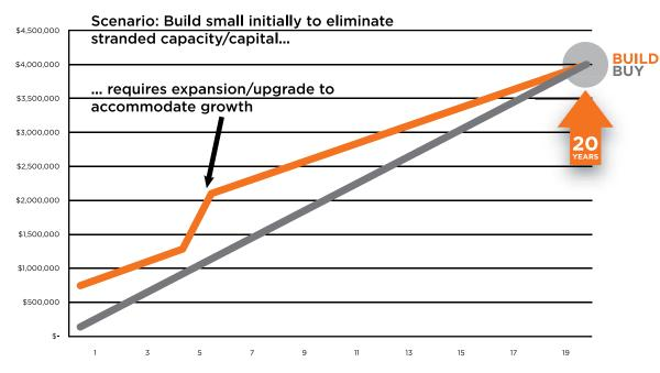
The utilization of a data centre changes over time and can range from 10% to 90%. Capacity, utilization, and the variation in utilization over time, are important factors to consider when performing a data centre TCO analysis to support a "Build vs. Buy" decision.
